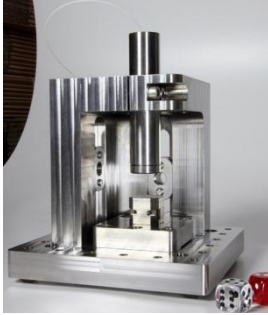
Figure 30: Interferometric setup for measurements of resonance frequencies
