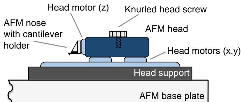
**Figure 3:** Schematic representation of the NeaSNOM probing head.
