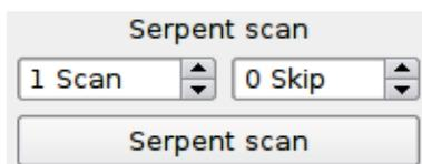
Serpent scan allows for coarse mapping of the specimen surface by performing a quick scan using a serpent-like pattern.
