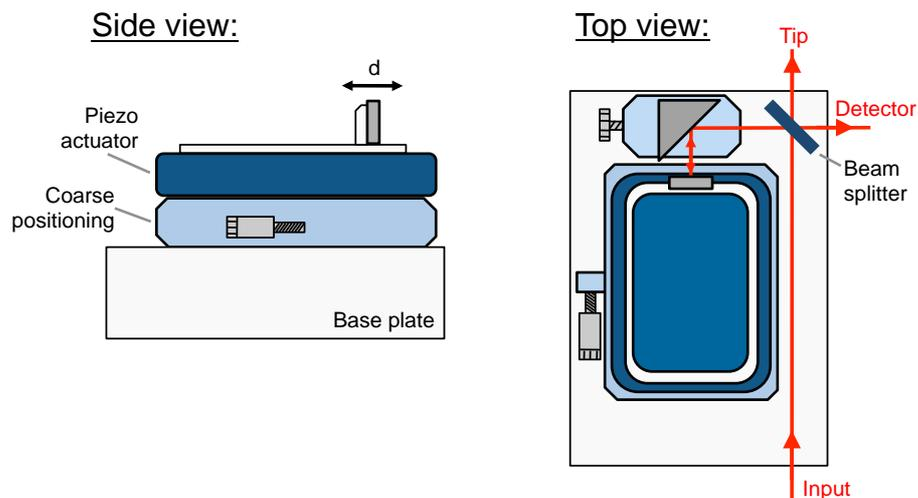
**Figure 13:** Schematic side and top view of the NeaSNOM broadband detection module.
