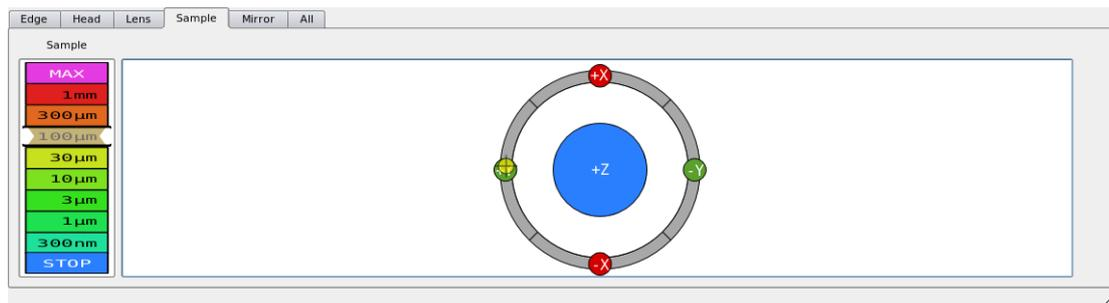
After selecting the tab with the part to be positioned, the motion speed needs to be adjusted. This can be done by rolling the mouse wheel or by clicking the desired speed indicator.
