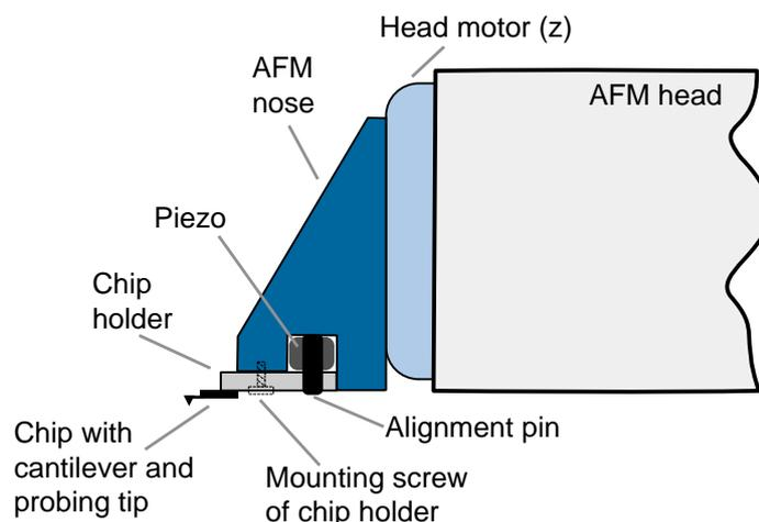
**Figure 4:** Sketch AFM nose with the cantilever chip holder.
