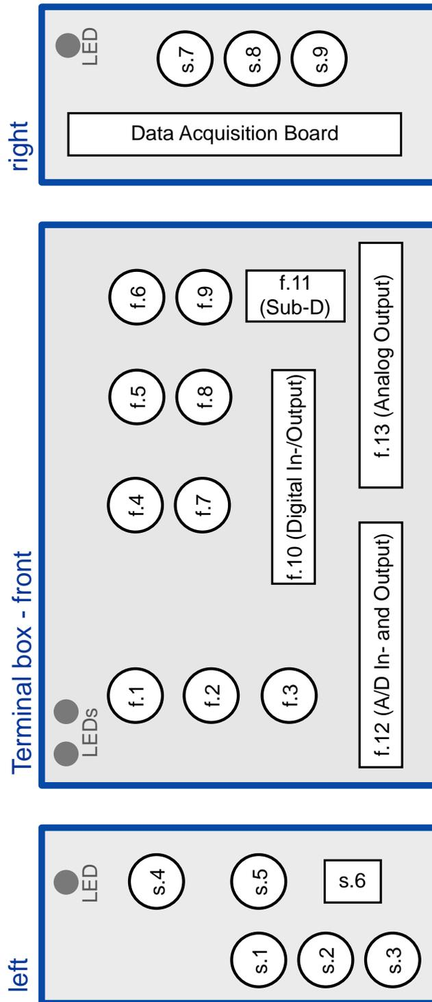
Figure 9: Sketch of the terminal box connectors.
