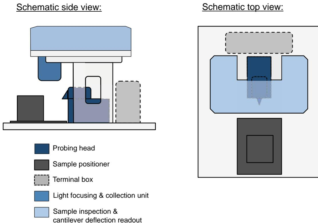
**Figure 2:** Side and top view (sketch) of the NeaSNOM microscope with the different units labeled.
