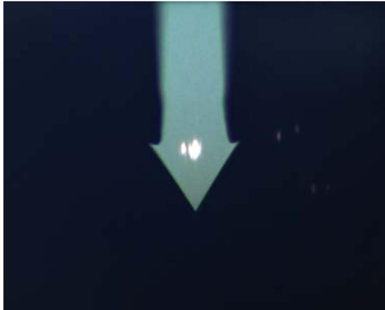
**Figure 6:** Image taken by the upright optical microscope showing a slightly elliptical focus of the deflection laser on a cantilever (Nanoworld, type ARROW™).
