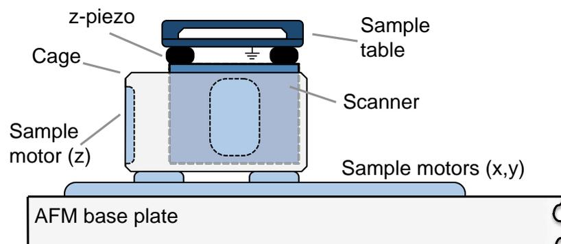
**Figure 7:** Sketch of the NeaSNOM sample positioner showing the coarse and fine positioning elements.
