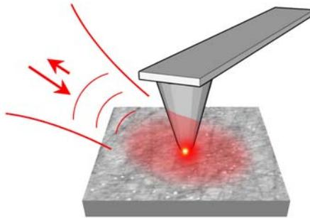
**Figure 1:** Basic principle of scattering-type Scanning Near-field Optical Microscopy (s-SNOM or ANSOM). The metalized probing tip of an AFM is illuminated by focused light and the back-scattered light is detected.
