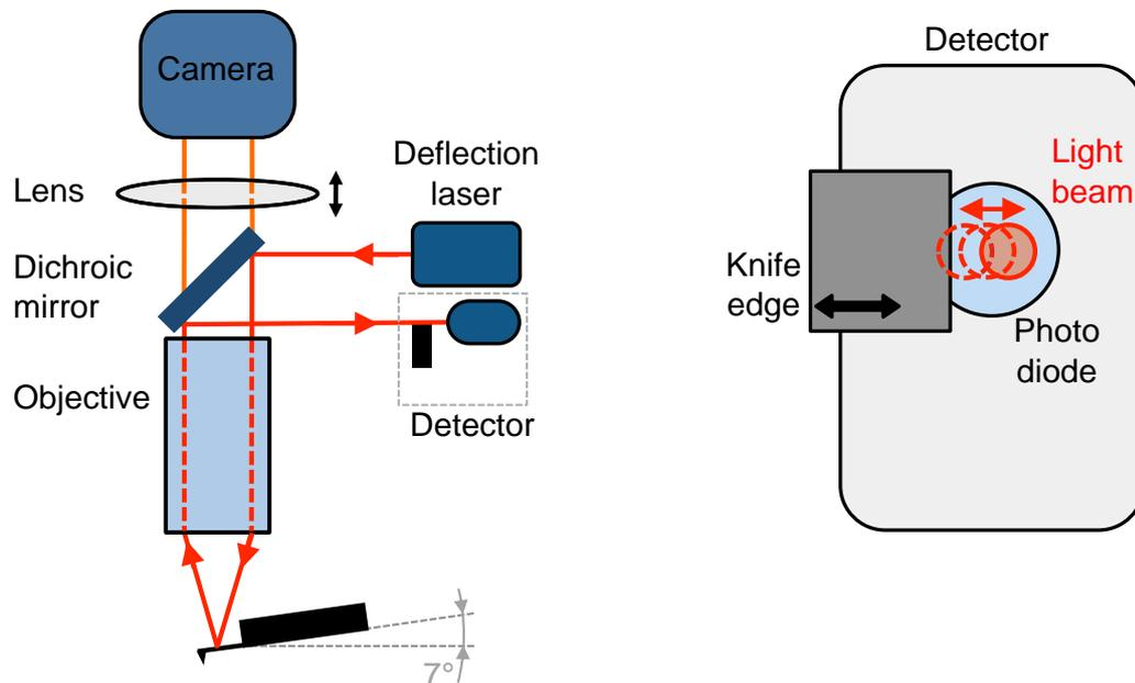
**Figure 5:** Optical beam path of the NeaSNOM sample inspection and cantilever deflection readout. The sketch on the right side shows the basic principle of the knife-edge detection method: the horizontally moving (oscillating) deflection beam is partly blocked, which results in a modulated electrical signal of the photodiode (see text for details).
