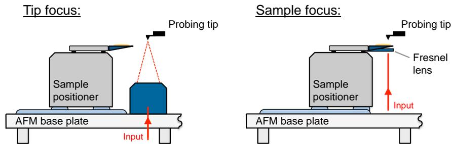
**Figure 14:** Transmission mode module of the NeaSNOM microscope with a fixed focal point at the position of the probing tip (left) or at a specific sample position (right).
