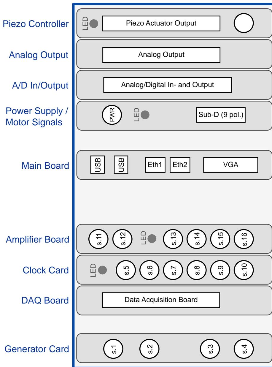
**Figure 8:** Sketch of the controller frontside with the individual boards and connectors labeled.
