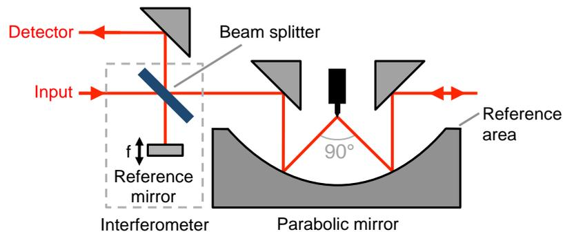
**Figure 10:** Optical beam path of the NeaSNOM microscope in the standard configuration.
