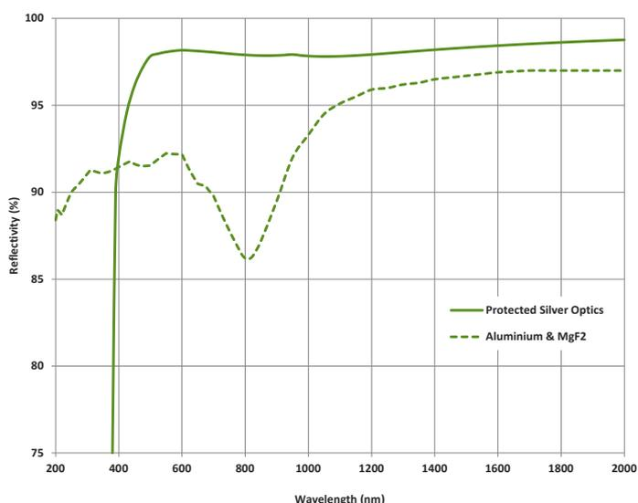
Standard systems use Al + MgF<sub>2</sub> coated optics. Protected silver optics are also available on request for maximum efficiency in the NIR region - recommended for working with Andor iDus InGaAs detectors or IR single-point detectors, such as MCT, PbS and InSb.
