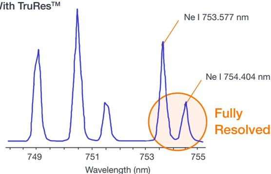
Kymera 328i with 300 l/mm grating, iVac 316 with high resolution 15 µm pixels, full vertical binning.
